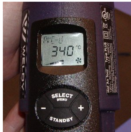
Set Temperature for the material type being welded.
