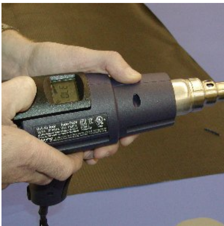
Set Temperature for the material type being welded.
