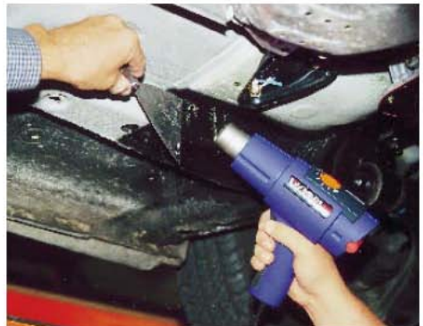
Removal of under-floor sealant
