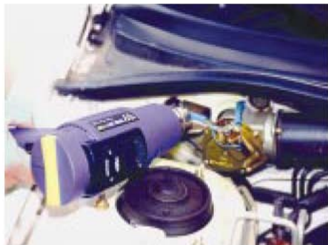
Shrinking a PVC heat-shrink tube.
