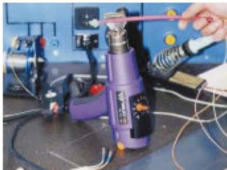
Shrinking a PVC heat-shrink tube with reflector.
