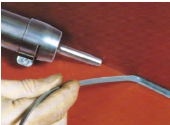
Pendulum welding of hard pvc with a 5 mm profile rod
