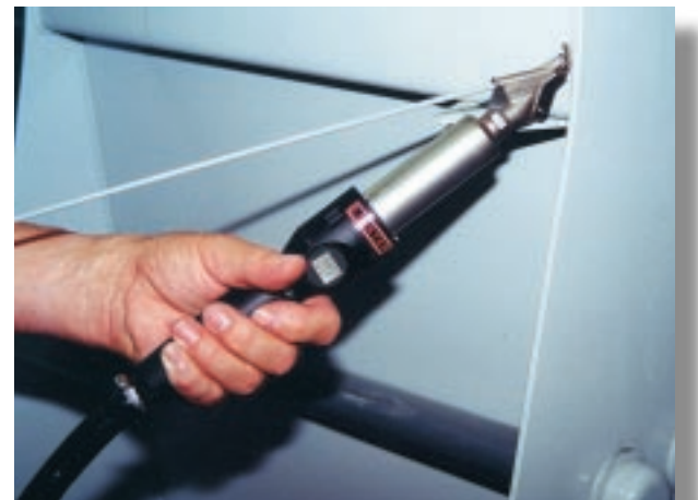
Welding PEN R with digital display for SET and ACTUAL value. The powerful welding tool.
