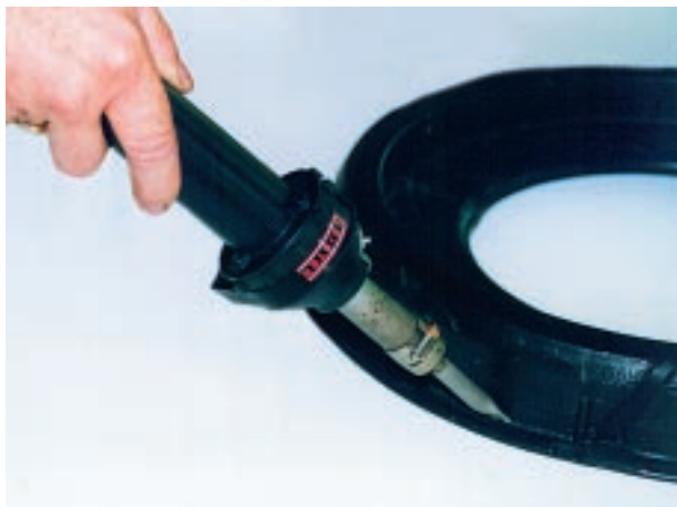
HOT-JET S being used for PE-HD tacking.
