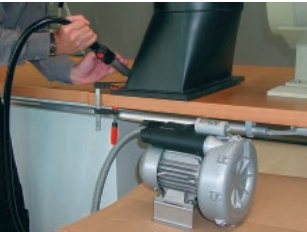
Welding PEN S the smallest and handy welding tool. Air supply from the high pressure blower ROBUST.
