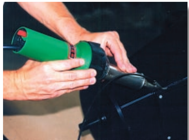
Welding of a PE-HD drum. TRIAC-S – the standard tool with high welding speed.
