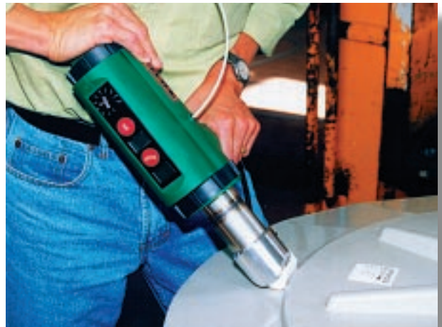
Weldmax Mini-Handextruder being used to weld PP
