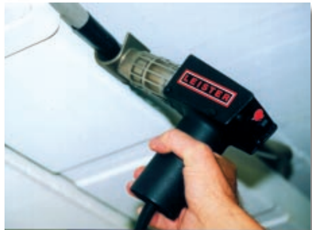
GHIBLI with sieve reflector for shrinking a PVC-tube.
